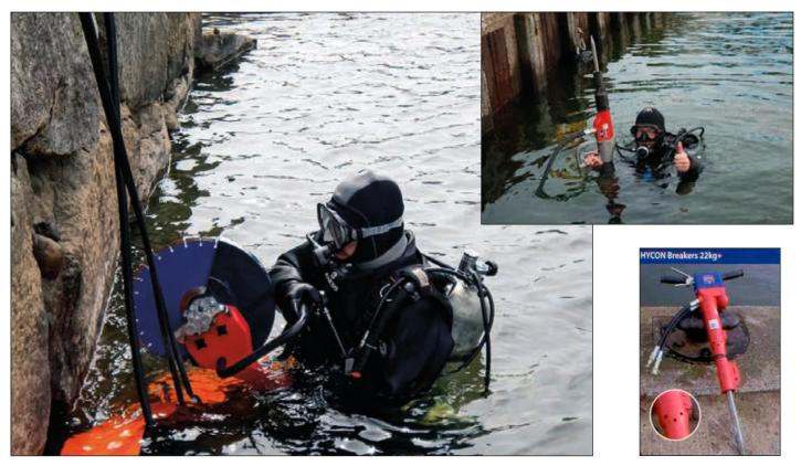
Most Hydraulic Hand Tools can be used underwater. Caution must be exercised on the Hydraulic Breakers to drill some relief holes prior to using underwater. Contact DITEQ Customer Service for specific details.
