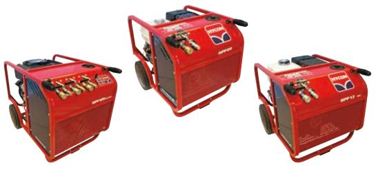
The **HPP06** is a 4.8GPM pack that is extremely simple (on/off) and can run most 5GPM tools. It is extremely portable (very compact and lightweight)
