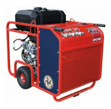
The HPP27VMF has Dual Pumps that combine for a full 16GPM flow or can be used on two different 8GPM tools. Some use a flow divided hydraulic circuit to approximate a dual even split of oil, whereby the HPP27 has two piggybacked individual pumps.
